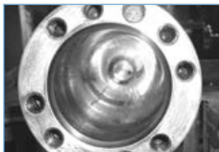
Scratches along the inside surface of a hydraulic cylinder reveal component damage caused by contaminants.
